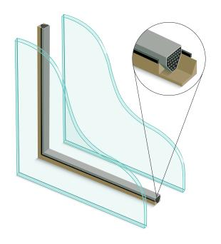
ur IG units are hermetically sealed combinations of two or more lites of glass separated by a dry airspace.
